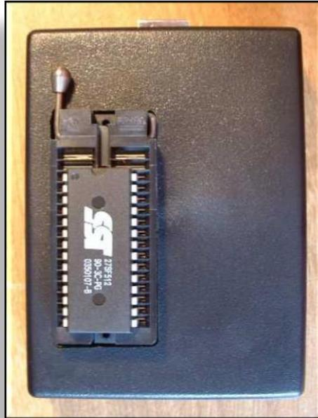
**Figure 1 – 28-pin Chip Orientation**
